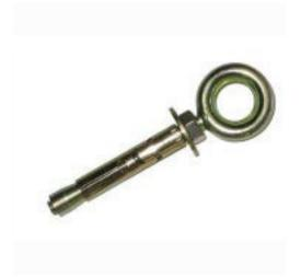
An overhead single-point fixing bolt. Ring size: 12mm Hole size required: 8-10mm x 50mm deep.
